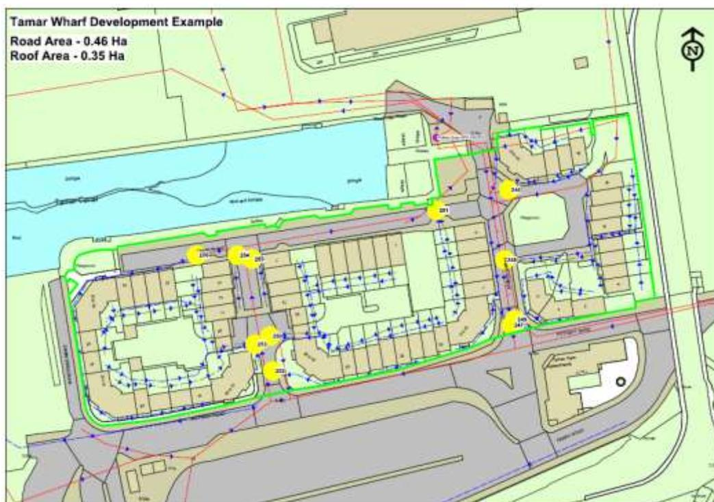
**Figure 3.1: Example of missed opportunity to discharge surface water to tidal waters as opposed to combined sewer system.**
